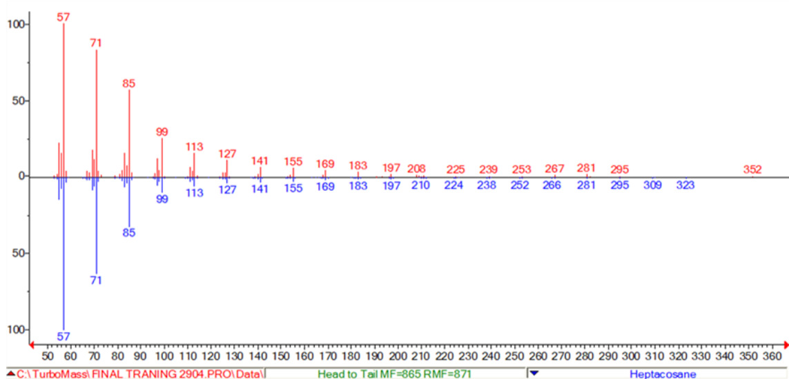
Fig. 14 The Head to Tail GCMS matching analysis of (Z)-13-Docosenamide and Heptacosane. As can be seen from the figure, the fragmentation patterns of the two compounds, a clear resemblance between the desired compounds and the standards used.
